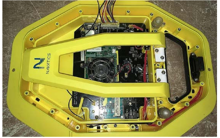
Inside the buoy. For cave use, the fan can be disconnected.
