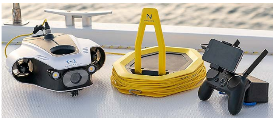
Components left to right: robot, buoy and control unit with smartphone.
