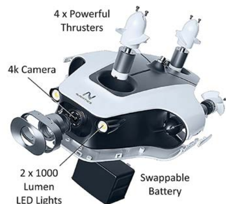
Exploded view of the Navatics Mito robot.
